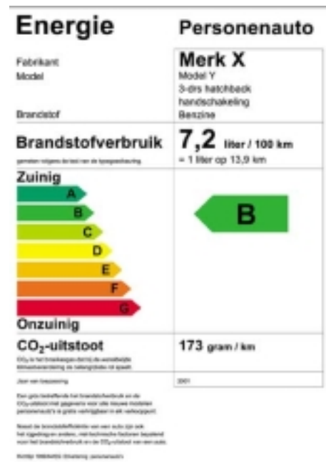
Figure 4: The Dutch label for fuel economy and CO 2 emissions for passenger vehicles.
