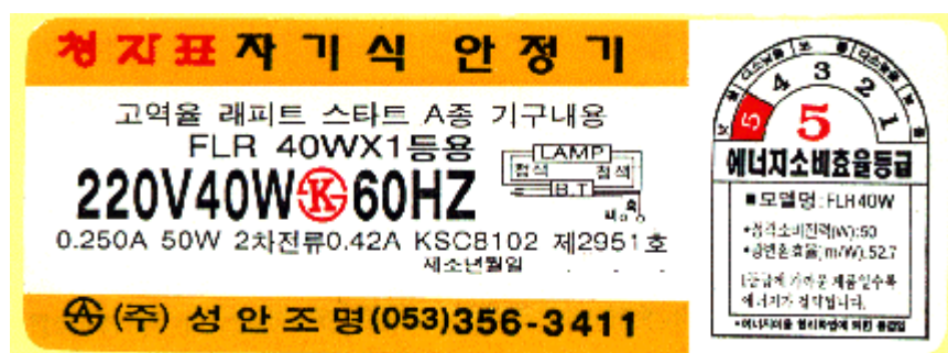
Figure 4. Energy label for a fluorescent ballast in the Republic of Korea
