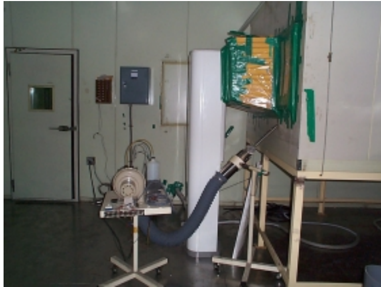
Figure 5. Testing in calorimeter room
