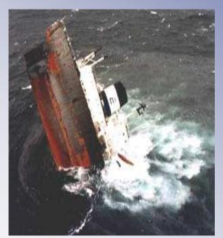
Tanker Erika, laden with 31,000 tons of heavy fuel, en route from Dunkirk (France) to Livorno (Italy) in very rough sea conditions was faced with structural problems off the Bay of Biscay. The Erika split in two and it sank the following day . Quantity spilled is between 19,000 and 20,000 tons.
