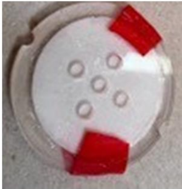
Fig. 9. GOES acrylic filter cartridge
