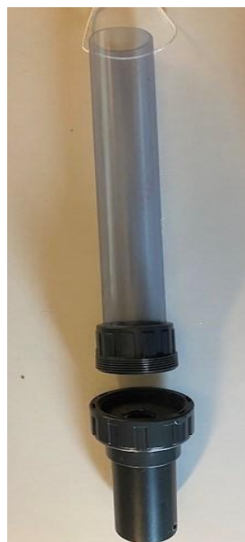
Fig. 7. GOES plankton sampler
