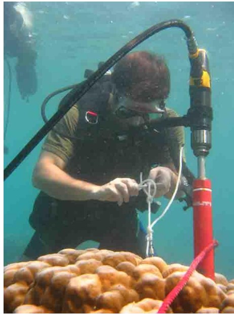
Core sampling from old coral rocks using Rock Corer
