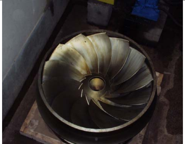
Figure 6: New runner for Tikvesh HPP
