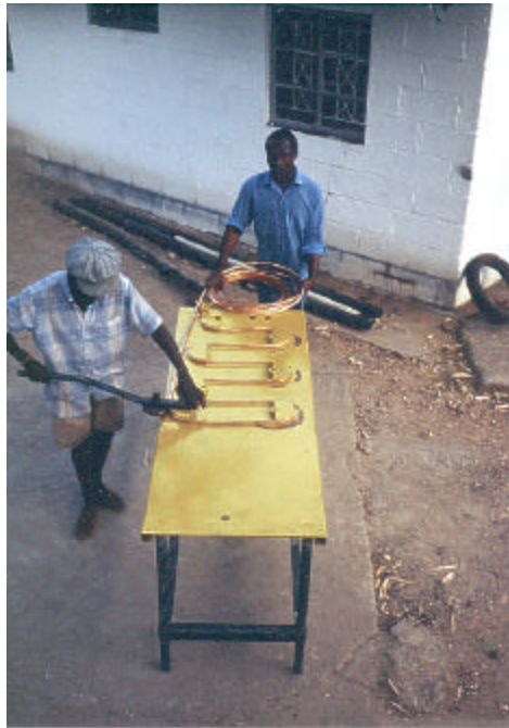
Fig. 2: Absorber manufacture using simple bending tools
