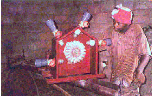
Figure 10: African village entrepreneur building a 4kW pico-hydro turbine, based on Sri-Lanka Technology, in Bapi village in Cameroon. Courtesy, IEPF project in Bapi.
