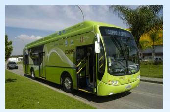
Hybrid Bus: Electricity and Hydrogen
