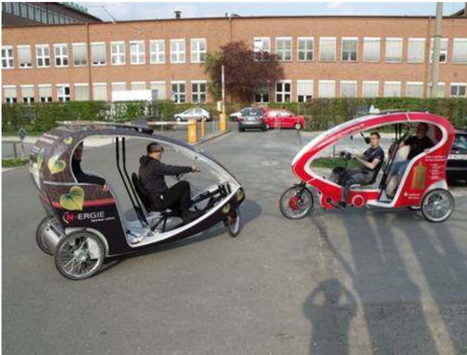
CCI (longer, wider) CCII (higher, suspension) new eVelotaxi 3600 Watt, 15% slopes (here with berlin`s mayor Klaus Wowereit)
