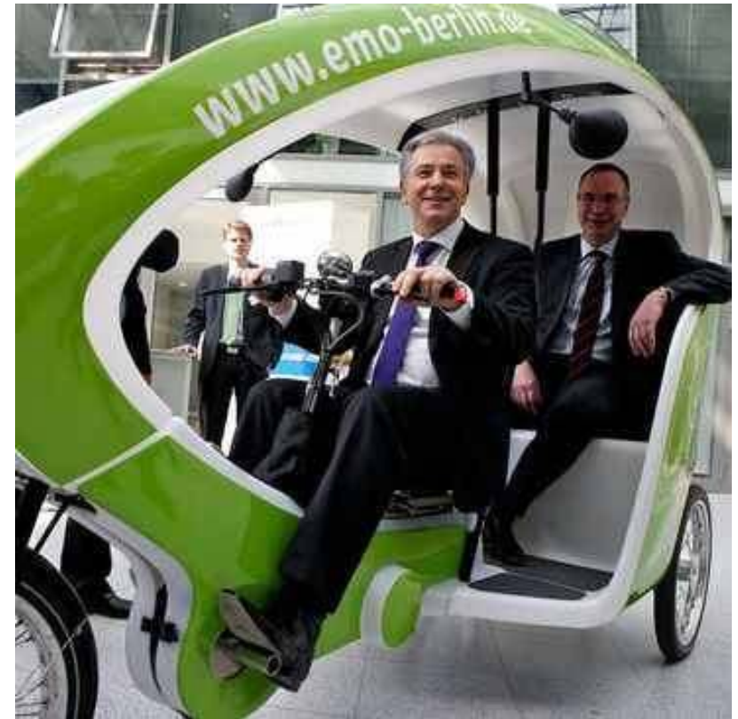
CCI (longer, wider) CCII (higher, suspension) new eVelotaxi 3600 Watt, 15% slopes (here with berlin`s mayor Klaus Wowereit)
