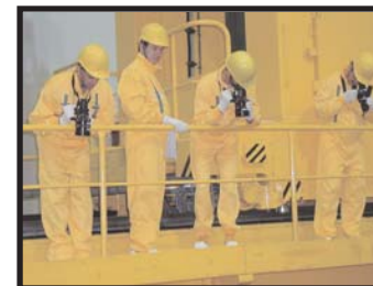
Inspectors employ a digitalized Cherenkov device at a nuclear fuel pond. A number of Member States conduct programmes to support the development of verification technology for use by IAEA inspectors. This piece of equipment was developed in order to help inspectors confirm that nuclear material is not diverted for the purpose of plutonium reprocessing.
