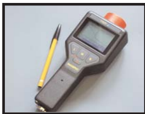
A hand-held radiation monitoring device. This monitor is a standard tool for spotting radiation. In the verification area, it may be used to confirm the presence of declared nuclear material or to detect any undeclared nuclear activities.
