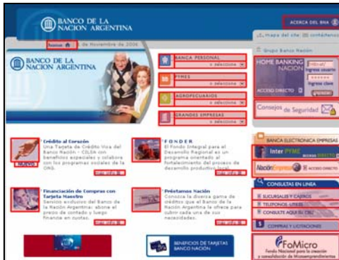
Figure 3: Images on the Bank of Argentina website with missing alternative text highlighted in red.
