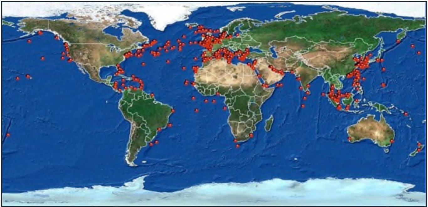
Figure 6. This distribution of 2,162 cable faults were recorded between 1959 and 2008 a period that covers the last of the telegraphic cables, coaxial cables and fibre-optic systems, the latter coming to prominence in the late 1980s. Most faults occurred in the shallow (<200 m deep) seas around Europe, SE Asia and eastern seaboard of North America and reflect the intense fishing and shipping activity of those regions. Faults across the North Atlantic Ocean result from the failure of old cables due to abrasion and component failure. For the rest of the BBNJ, cable faults are presently 4 per annum worldwide 59 . (Figure used with permission of TE Subcom.)
