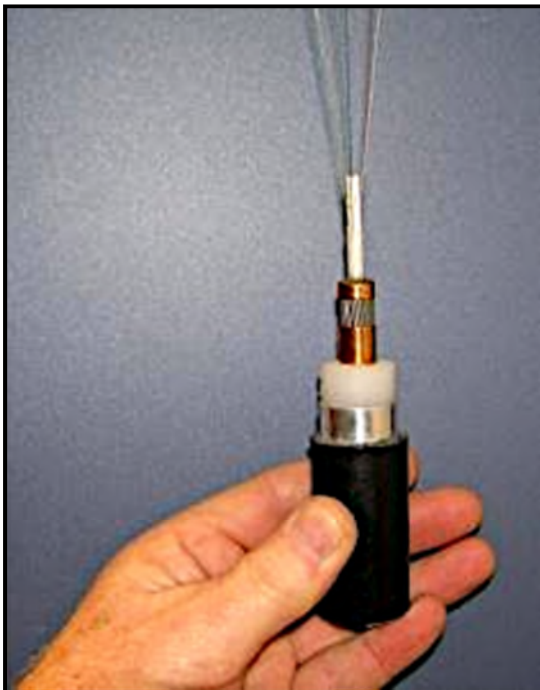
Figure 5. A lightweight fibre-optic cable with (from outside to core) black and white polyethylene sheath, power conductor (copper), wire strength member, glass fibres and plastic support sheath (white).
