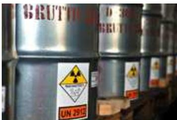
Uranium ore is processed into a concentrate known as yellowcake and packed in special, tightly sealed steel drums similar in size to oil barrels. Photo: IAEA
